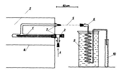
Fig. 1. Gas chromatograph adapted to the sweep codistillation cleanup. 1-Modified Storherr tube packed with Pyrex glass wool. 2-Detector oven of the gas chromatograph. 3-Injection type septum. 4-N<sub>2</sub>-inlet. 5-Connection for the condenser with the Sorherr tube. 6-Condenser. 7-Openings in the wall of the detector oven. 8-A wall between the detector and column ovens of the chromatograph. 9-Ice bath. 10-Graduated collection tube.
